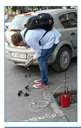
Once the leak has been identified, the PCorr+ devices can be easily extracted and moved to other areas within the network to continue looking for leaks.
